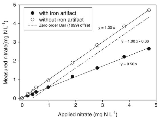
**Fig. 1** Adsorption isotherm of  $\text{NO}_3^-$  in Harvard Forest organic soil. Closed circles (●) represent samples measured with iron artifact; open circles (○) represent samples measured without iron artifact. Measured  $\text{NO}_3^-$  concentrations are corrected for background  $\text{NO}_3^-$  which was measured as 0.8 and 1.1 for samples as measured with iron artifact and without iron artifact, respectively
